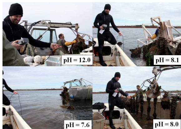
Figure 3. DFARD staff measuring pH at varying distances from a liming operation. Clockwise from top left: tank with lime solution, 1 m away from application site, 3 m away from application site, and greater than 10 m away from application site.
