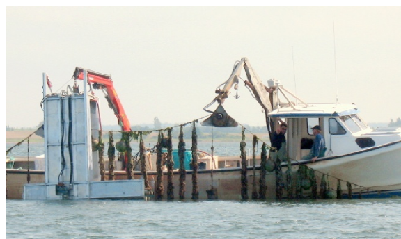
Figure 2. Lime spray system being used to control clubbed tunicate, S. clava , fouling on mussel socks.
