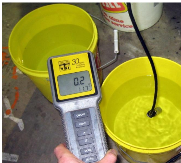
Figure 4. Experimental units were fully immersed in fresh water for a predetermined exposure.
