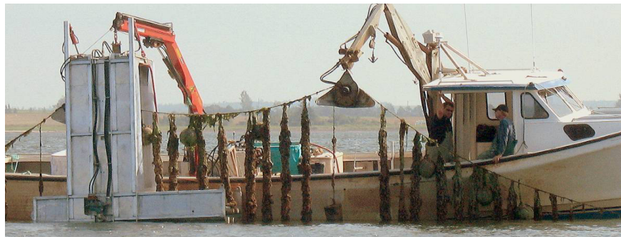
Figure 5. Lime spray system being used to control clubbed tunicate, S. clava , fouling on mussel socks.
