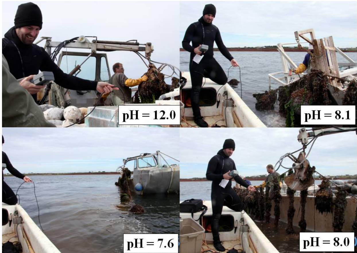
Figure 7. DFARD staff measuring pH at varying distances from a liming operation. Clockwise from top left: tank with lime solution, 1 m away from application site, 3 m away from application site, and greater than 10 m away from application site.
