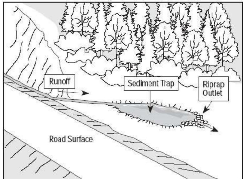
Both need regular cleaning with a backhoe and require frequent and on-going maintenance.
