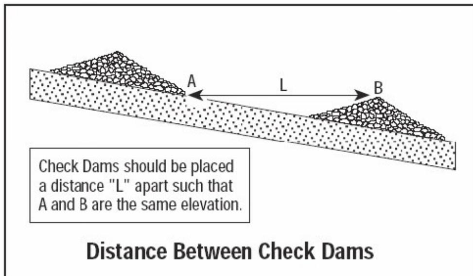
Figure 3 – Distance requirements between check dams
