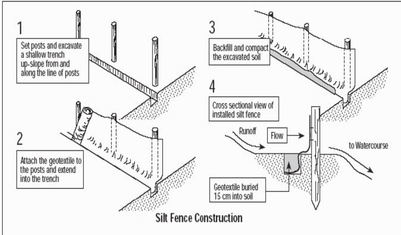
Figure 4 – Silt Fence Construction
