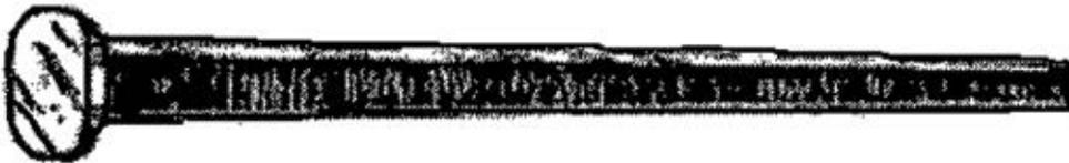
Cut nails taper on only two sides of their shanks, and the cut sides usually show marks from the cutting machine.
