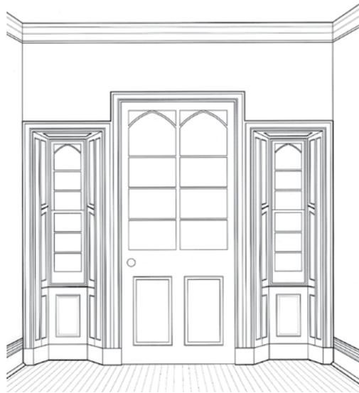
A transom window was often installed above the door to let light and air into the entry on the other side. If the entry hall was wide enough, the door could also feature sidelights on either side.
