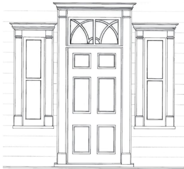
Doors were traditionally made of wood and assembled much like a window. Panels and sometimes window glass were set into a framework of rails and stiles. The resulting door was light but strong and durable. Like windows, the way a door was built made it look like it did.
