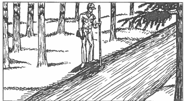
Fig. 16 Use a rod to assess foundation conditions.
