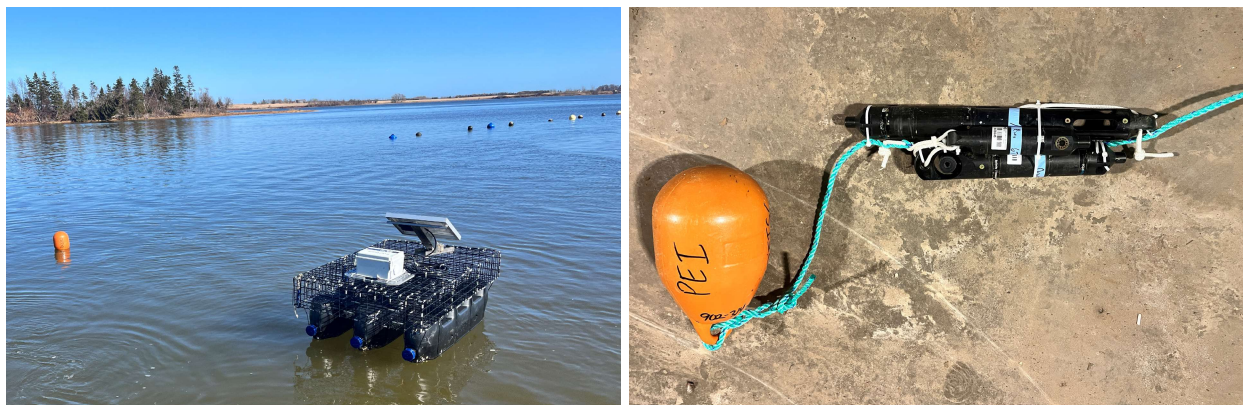
Figure 12. Innovasea Live Data Platform ( left ) and associated water quality instruments ( right ).
